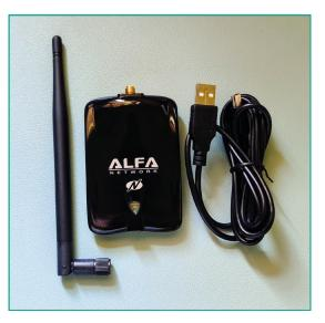
Figure 7.23 – Alfa AWUS036NHA wireless network adapter
