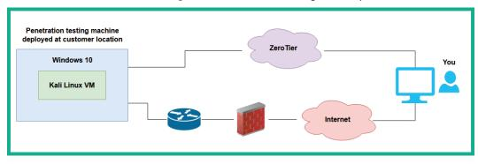
The following diagram provides a visual representation of a penetration tester's machine at a client's location with the actual penetration tester working remotely.
