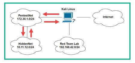
Figure 9.21 – Penetration testing lab topology
