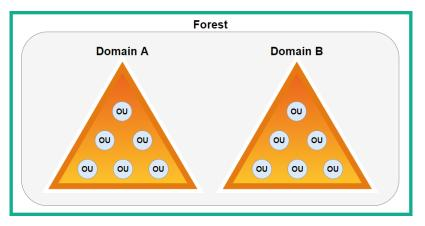
The following diagram shows the structure of a forest with multiple domains:
