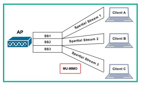
The following diagram provides a visual representation of MU-MIMO:
