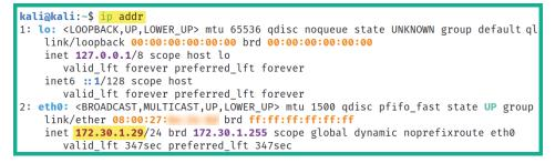
Figure 7.5 – Determining the IP address
