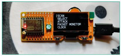
Figure 17.2 – ESP8266 microcontroller
