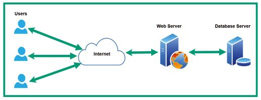
The following diagram shows a visual representation of a web server deployment:
