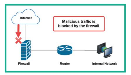
Figure 5.31 - Network-based firewall
