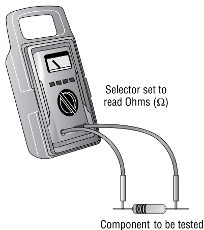
FIGURE 1.22 Connecting a multimeter to measure resistance
