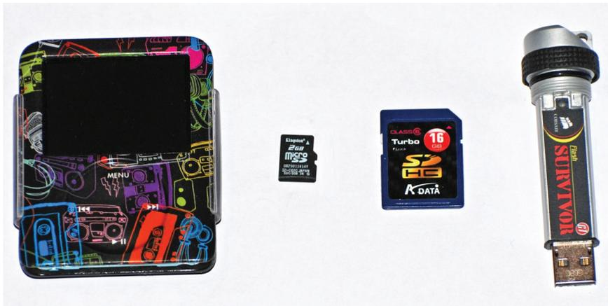
A *removable device* or drive is a storage device that is designed to be removed from the computer without turning the computer off. These devices range from the MicroSD memory card, which is the size of a fingernail and can store 32 GB (or more) of information, to an external hard drive, which can store up to 4 TB of data. CDs, DVDs, and USB drives are also considered removable drives, because they can be used to store critical data and are easily transportable.
