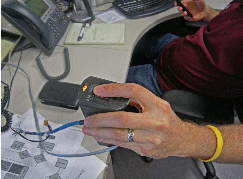
To initially use the biometric system, set up an enrollment station where an administrator enrolls each user, which includes scanning the biometric feature to be used for authentication. When selecting a biometric method, consider its performance, difficulty, reliability, acceptance, and cost. In addition, look at the following issues:
