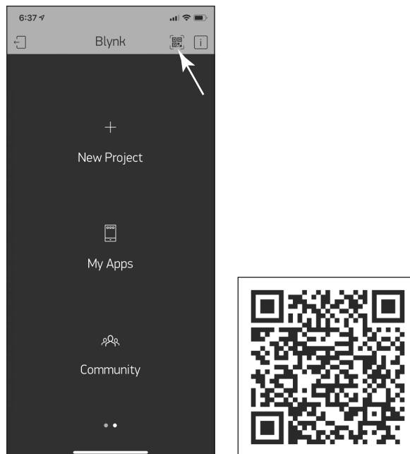
FIGURE 3-12: Click for QR (left), and then scan the QR to generate your myTemperature app in Blynk.
