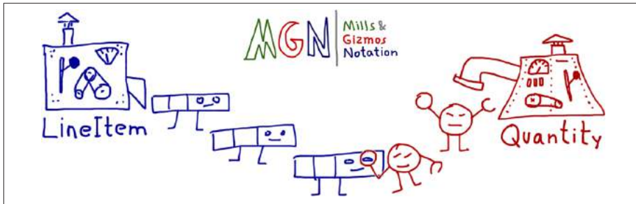
Figure 20-3. MGN sketch showing the LineItem class making three instances, and Quantity making two. One instance of Quantity is retrieving a value stored in a LineItem instance.
