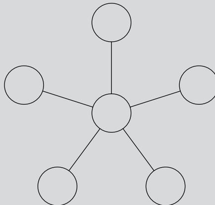
In a star network, all the nodes are connected to a central hub. In effect, each node has an independent connection to the network, so a break in one cable doesn't affect the others.
