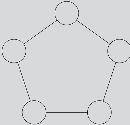
A ring is very much like a bus except with no end to the line: The last node on the line is connected to the first node, forming an endless loop.
