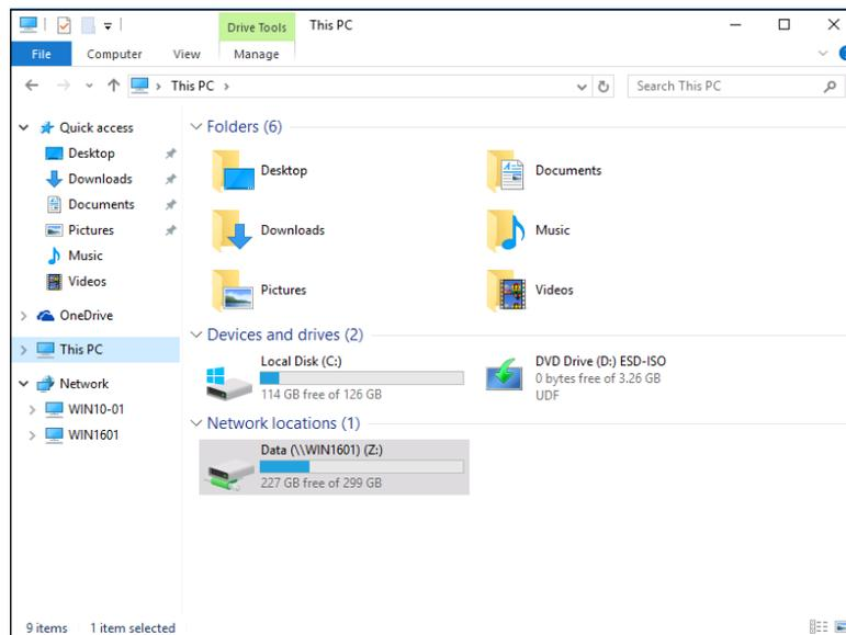
**FIGURE 3-6:** The This PC folder shows a mapped network drive.
