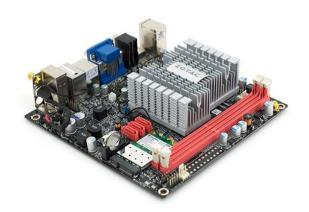
The motherboard of an HTPC usually doesn't have much impact on performance, but it's still important. Why? Because the motherboard determines the connectivity available, and it's also usually the largest component – which means it dictates how compact your HTPC can be.
