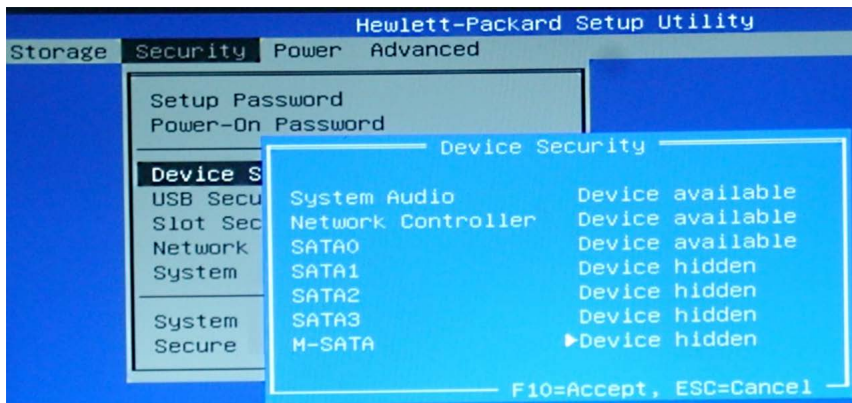
Figure 16.14: Disabling drive ports on my Hewlett-Packard Envoy
