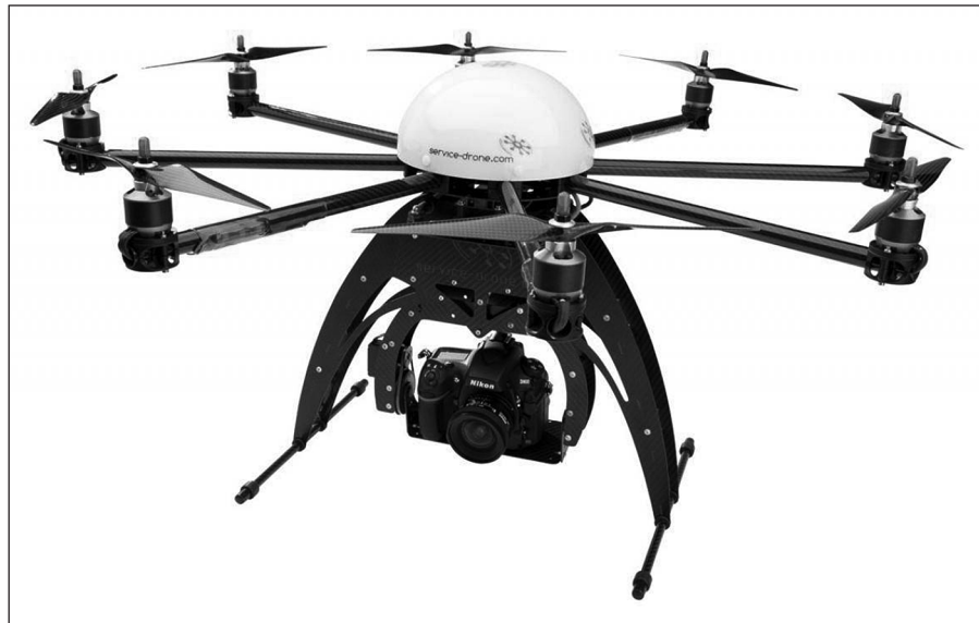
Figure 3-2: Octocopters have 8 propellers.
