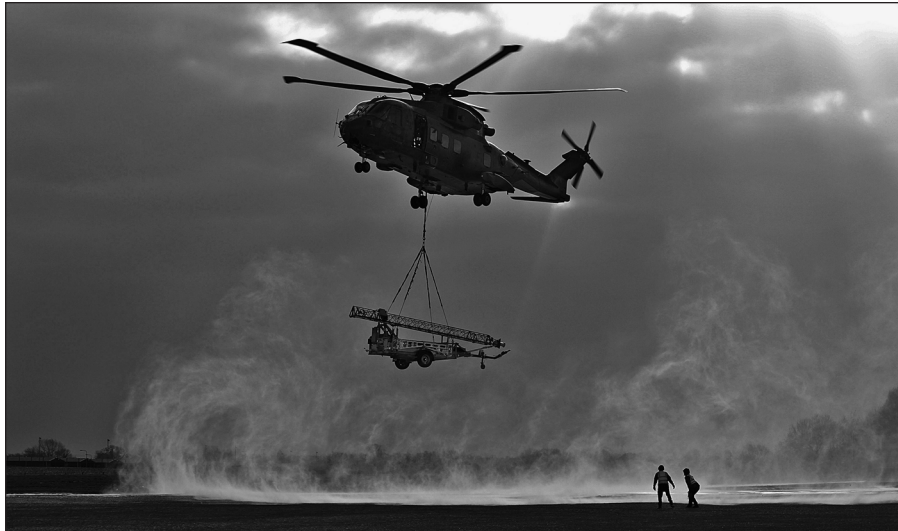
Figure 9-9: Ground wash can cause unman- ageable turbulence if you aren't careful.
