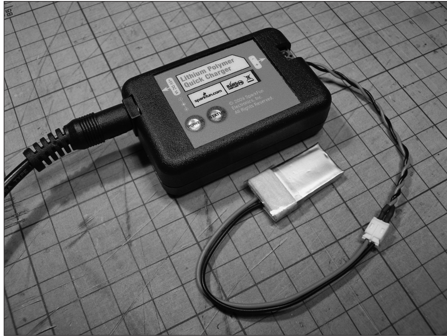
Figure 5-8: Drone battery chargers look the same but may be different.
