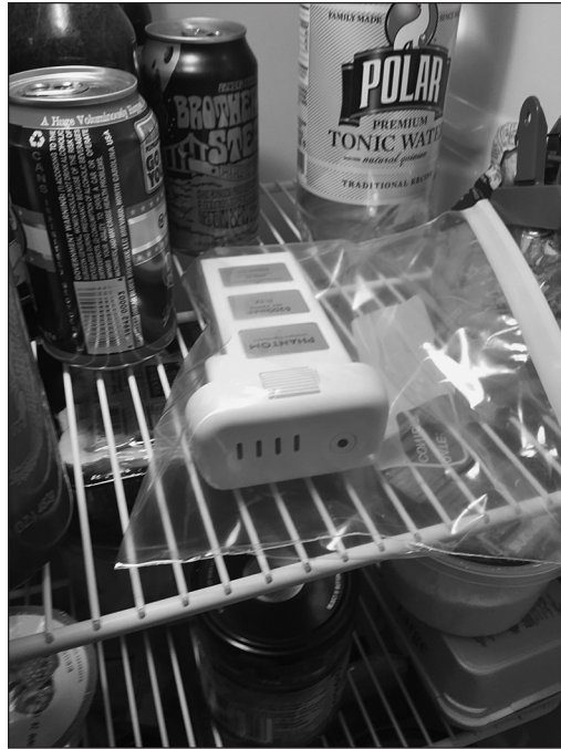
Figure 11-10: Safely storing LiPo batteries in a refrigerator.
