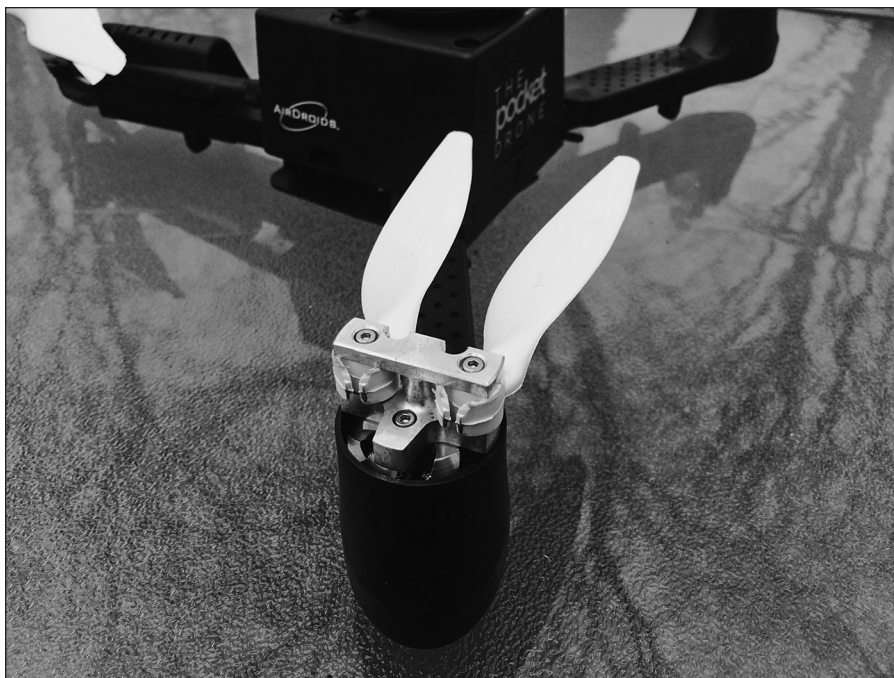
Figure 11-6: Fittings are screws and washers that keep drone parts secure.
