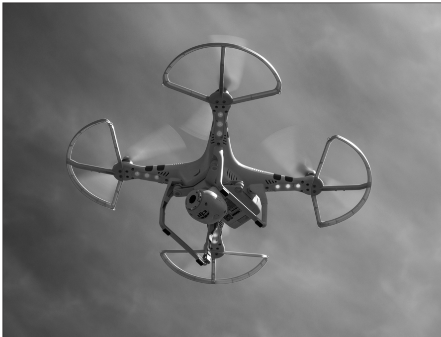
Figure 6-2: Propeller guards will pro- vide some protection from spinning propellers.
