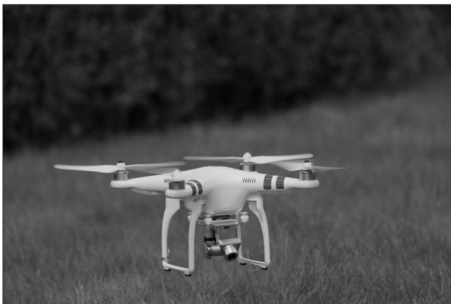
Figure 5-3: The DJI Phantom 2 airframe is designed to protect its electrical components like the computer and navigational sensors.
