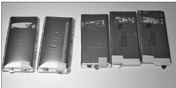
Figure 11-5: Damaged LiPo batteries are hazardous to your health.
