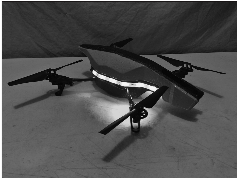
Figure 10-6: Night flying is possible with down- ward lights.
