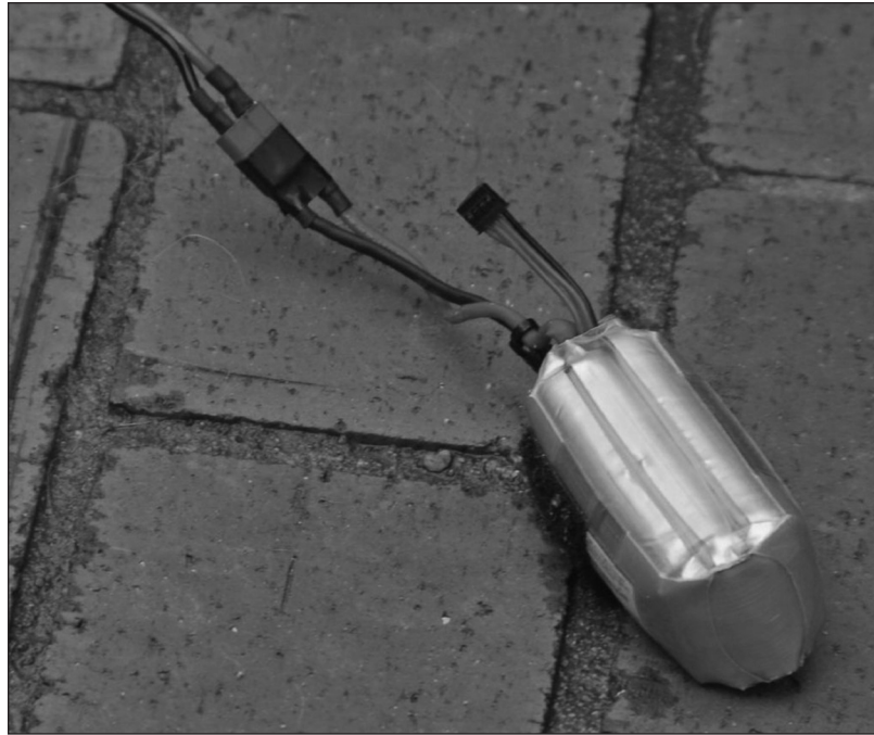
Figure 6-6: Bury swollen LiPo batteries in a bucket of sand.
