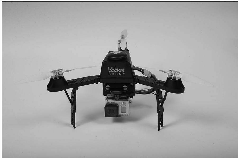
Figure 5-11: Mount your go pro to a pocket drone with adhesive.
