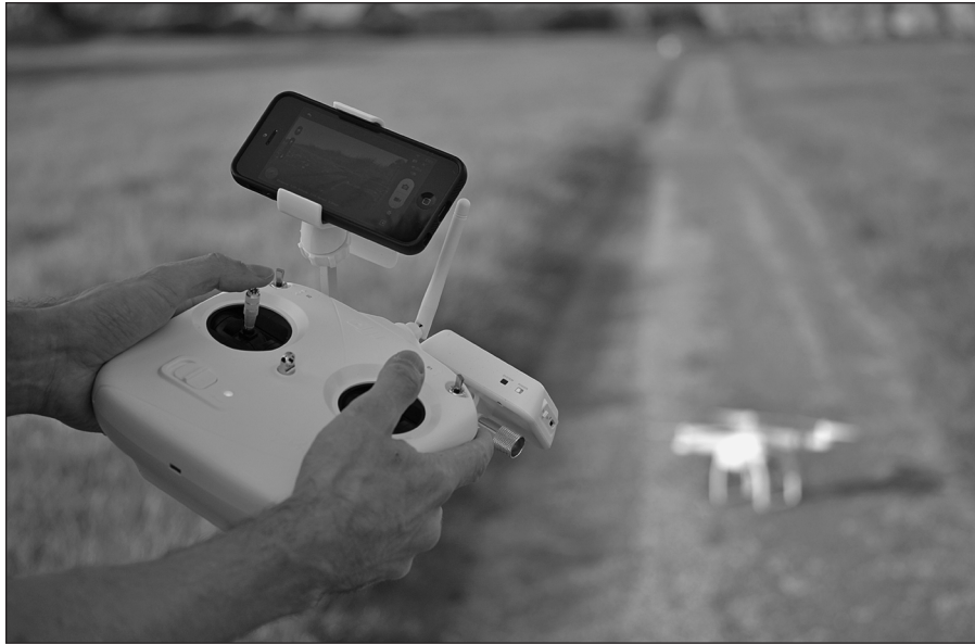
Figure 8-4: The DJI Phantom 2 remote control uses RF.
