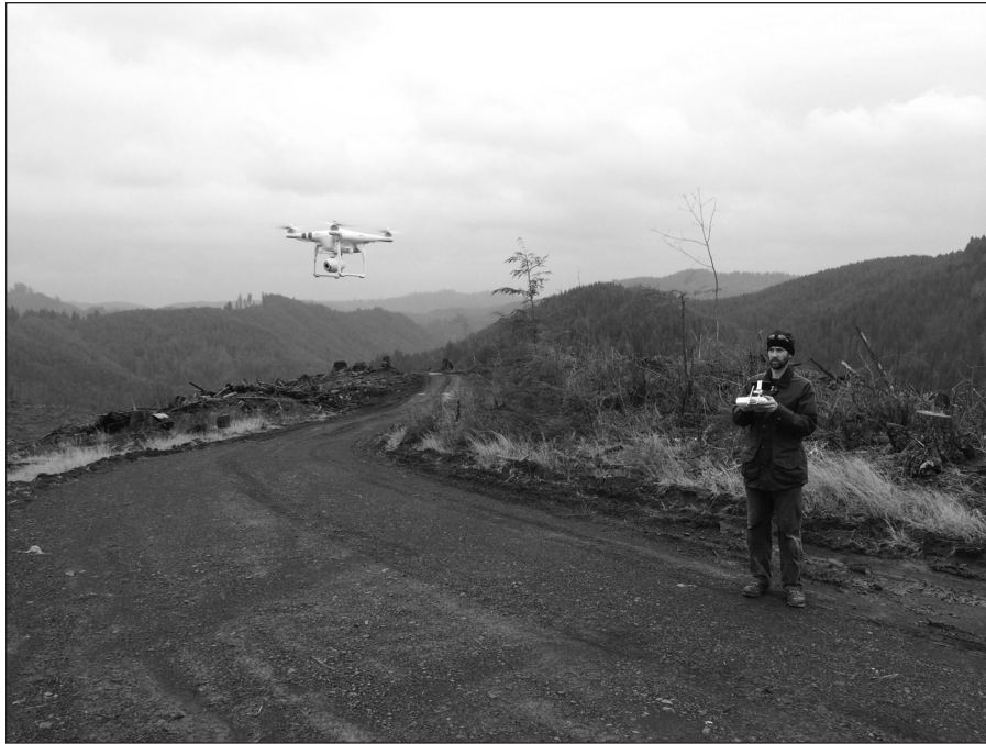
Figure 9-4: Use your body as a reference for how high to hover your drone to verify stability.
