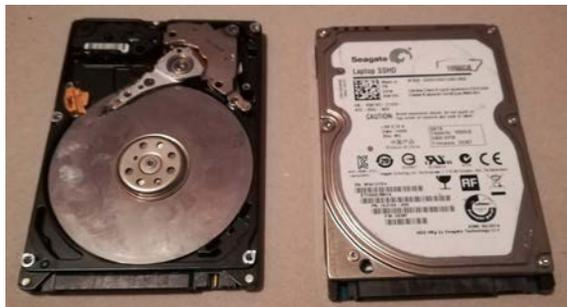
Figure 3.8 – A mechanical laptop drive with platters exposed
