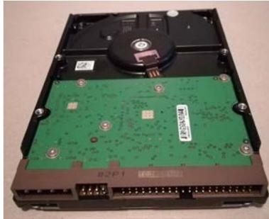
Figure 3.6 – An older 40-pin EIDE hard disk drive
