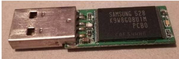
Figure 3.1 – A flash drive with the NAND chip exposed
