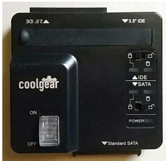
Figure 4.7 – Portable Coolgear Write Blocker
