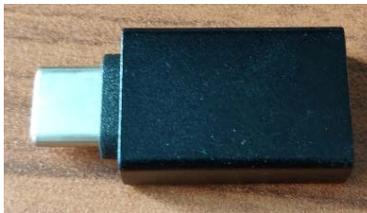
Figure 4.6 – USB to USB type-C adapter
