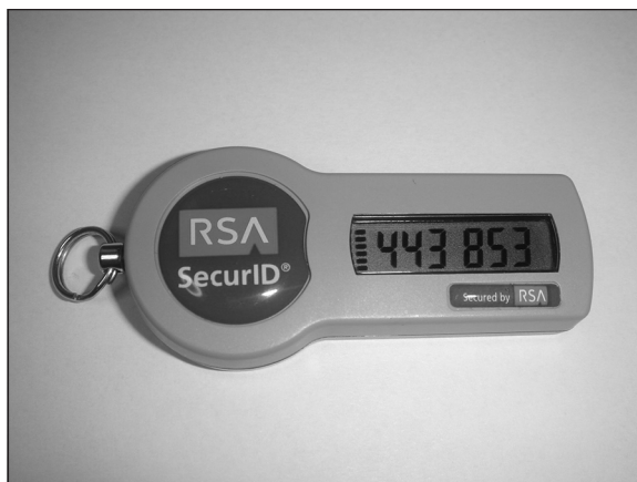
FIGURE 5-4: An RSA SecurID brand one-time password generator hardware token.
