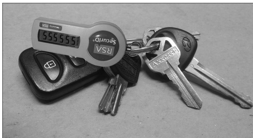
FIGURE 6-1: Fobs, often placed on keyrings, provide one-time tokens without the need for a mobile phone.
