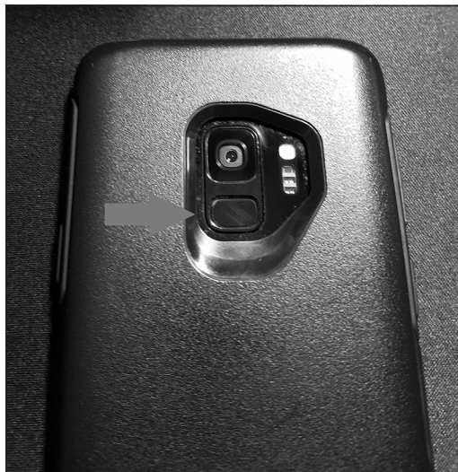
FIGURE 5-3: A phone fingerprint sensor on a Samsung Galaxy S9 in an OtterBox case. Some phones have the reader on the front, while others, like the S9, have it on the back.
