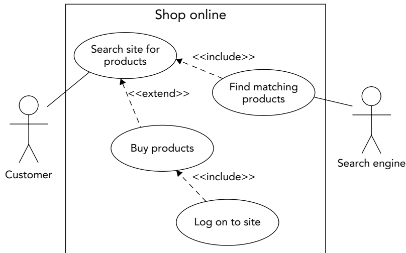
FIGURE 6.11: A use case diagram shows actors and the tasks they perform (possibly with subtasks and extensions).
