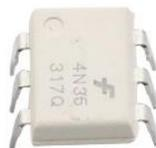
The 4N35 is an optocoupler for general purpose application. It consists of gallium arsenide infrared LED and a silicon NPN phototransistor.
