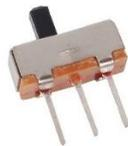
A slide switch, just as its name implies, is to slide the switch bar to **connect** or **break** the circuit, and further switch circuits. The common-used types are SPDT, SPTT, DPDT, DPTT etc. The Slide Switch is commonly used in low-voltage circuit. It features flexibility and stability, and widely applies in electric instruments and electric toys.
