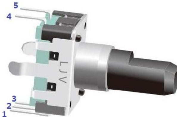
A rotary encoder is an electronic switch with a set of regular pulses with strictly timing sequence. When used with IC, it can achieve increment, decrement, page turning, and other operations such as mouse scrolling, menu selection, and so on.
