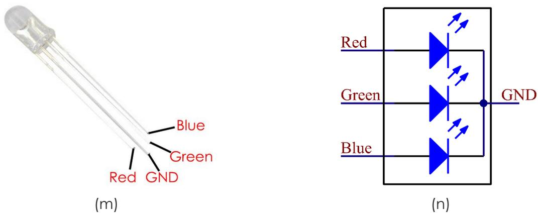
An RGB LED has 4 pins: the longest one is GND; the others are Red, Green and Blue. Touch its plastic shell and you will find a cut. The pin closest to the cut is the first pin, marked as Red, then GND, Green and Blue in turn.
