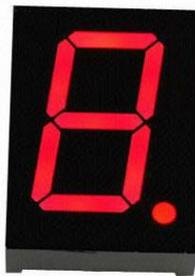
Each of the LEDs in the display is given a positional segment with one of its connection pins led out from the rectangular plastic package. These LED pins are labeled from "a" through "g" representing each individual LED. The other LED pins are connected together forming a common pin. So by forward biasing the appropriate pins of the LED segments in a particular order, some segments will brighten and others stay dim, thus showing the corresponding character on the display.
