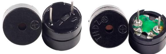
The difference between an active buzzer and a passive buzzer is: An active buzzer has a built-in oscillating source, so it will make sounds when electrified. But a passive buzzer does not have such source, so it will not beep if DC signals are used; instead, you need to use square waves whose frequency is between 2K and 5K to drive it. The active buzzer is often more expensive than the passive one because of multiple built-in oscillating circuits.
