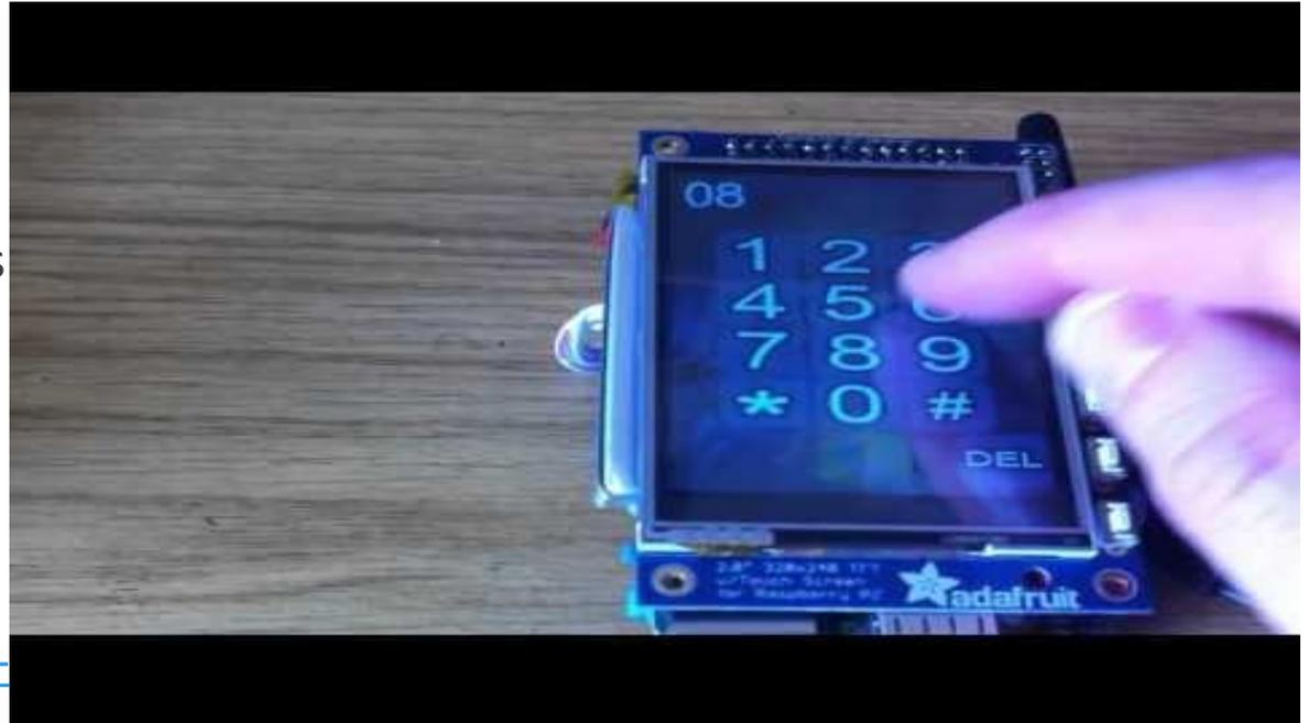
Video showing a smartphone made with Raspberry Pi .
