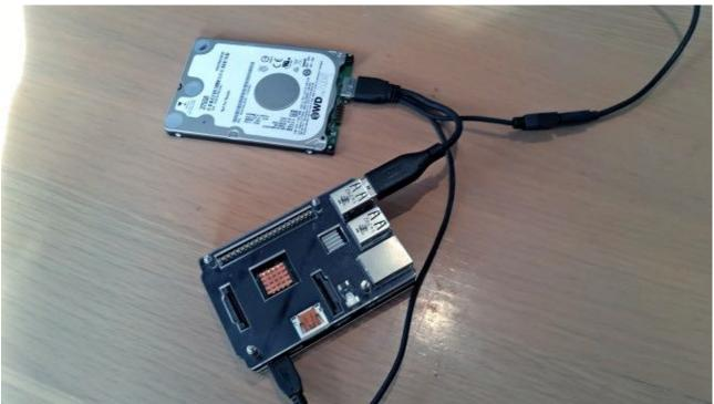
One option is to purchase a **PiDrive**, a hard disk produced by Western Digital. This ships with a custom version of NOOBS (see below), enabling you to install multiple Pi operating systems onto a 375 GB or 1 TB HDD. The advantage to this is that you don't have to install a new OS each time you need to start a new project.
