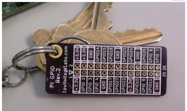
Although detailed use of the GPIO pins is beyond the scope of this guide, safety isn't. You will need to adopt the same careful approach to connecting to these pins as you would on any computer or circuit board. Without proper care, you risk blowing up your Raspberry Pi's CPU if the GPIO pins are used incorrectly. Make sure you test the voltage through the cable before connecting to your Pi!
