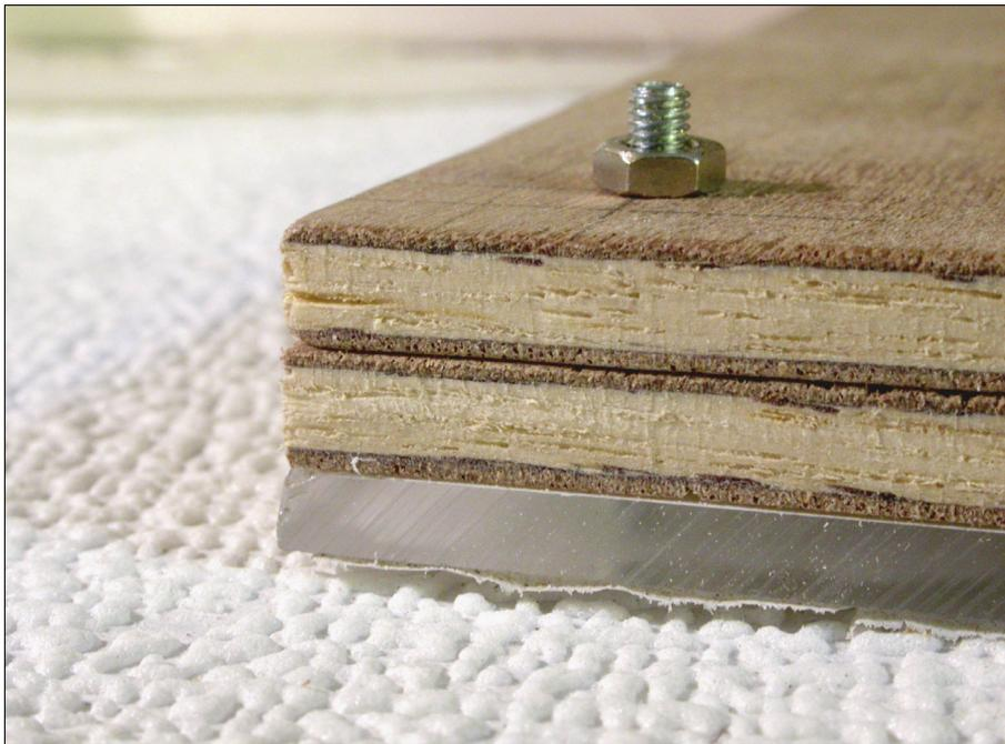
To make the top frame, do exactly the same thing that you did to create the bottom tray, except using 17mm (11/16") strip pine. When this is set, glue it into a piece of 2mm (3/32") foam from a hobby or card-making shop or office-supply store. You can then cut the foam to size on the inside and outside of the frame using a sharp knife. In that way, you get a neat gasket that looks good through the acrylic and helps bed things down.
